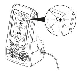
⇒ The device switches on automatically as you connect the charging cable and a charging indicator will appear on the display.
